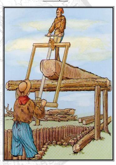
Before the days of water-powered lumber mills, two men working as a team cut beams and boards for house and ship construction.
